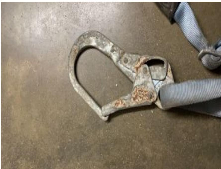
**Safe? Not a chance!** This corroded snap hook was removed from service during a recent inspection. According to the Occupational Safety and Health Administration "Personal fall protection systems must be inspected before initial use during each work shift for mildew, wear, damage, and other deterioration, and defective components must be removed from service."
